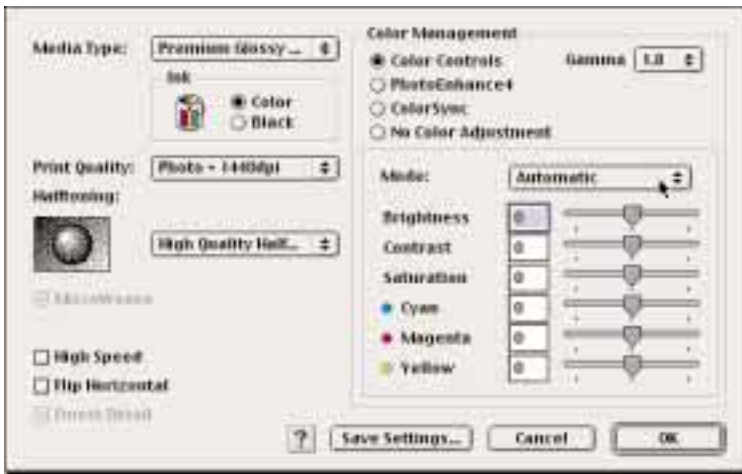
In the Advanced Epson dialog, set the Media Type for the paper you are using, Print Quality to PPhoto-1440 dpi, Halftoning to High Quality Halftoning, Color Management to COlor Controls - Automatic then choose Save Settings to save these settings for later selection from the regular print dialog.
